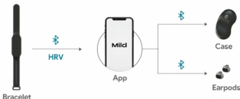
Figure 29: System Architecture
