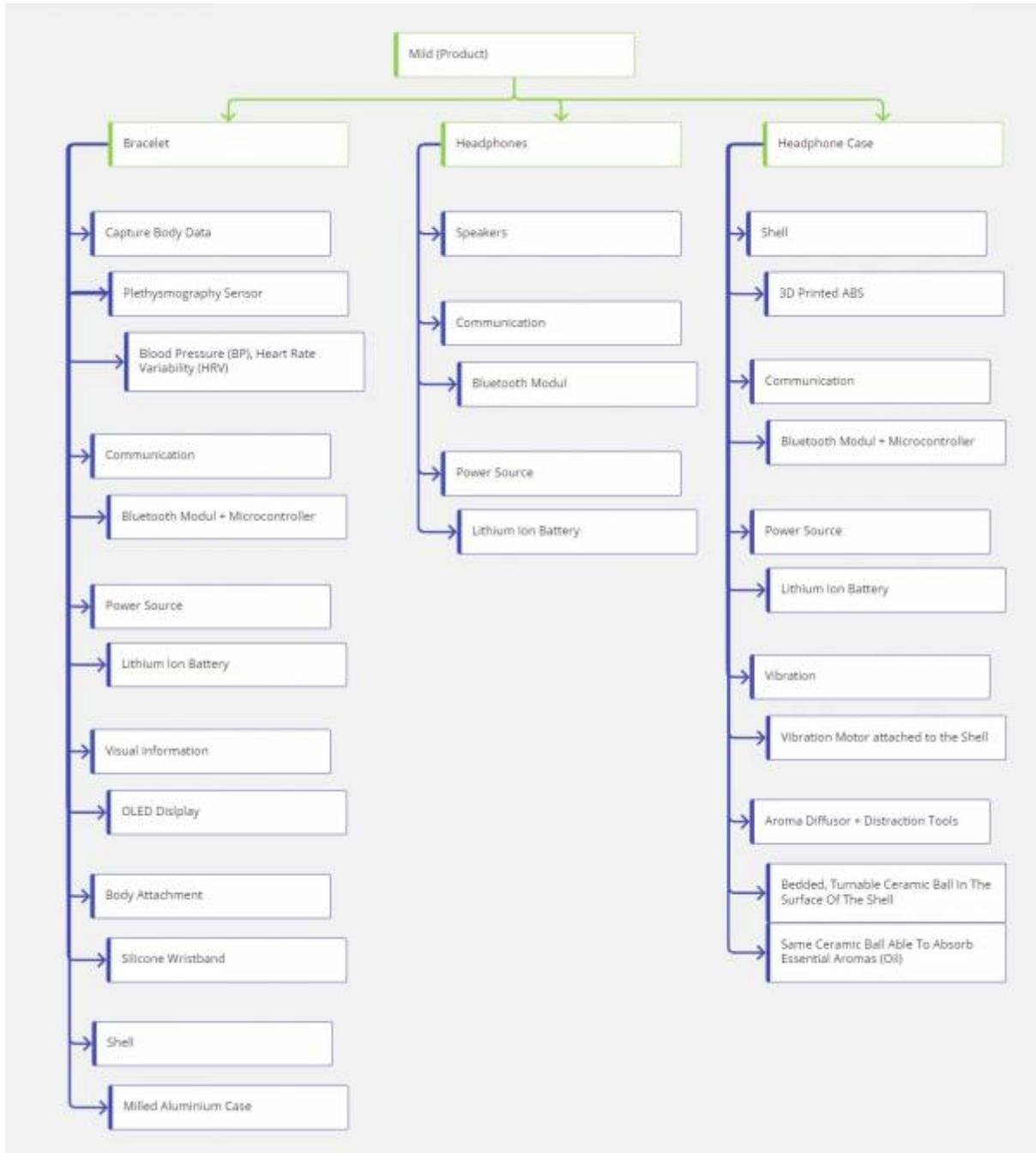
Figure 12: Work Breakdown Structure of Product Scope
