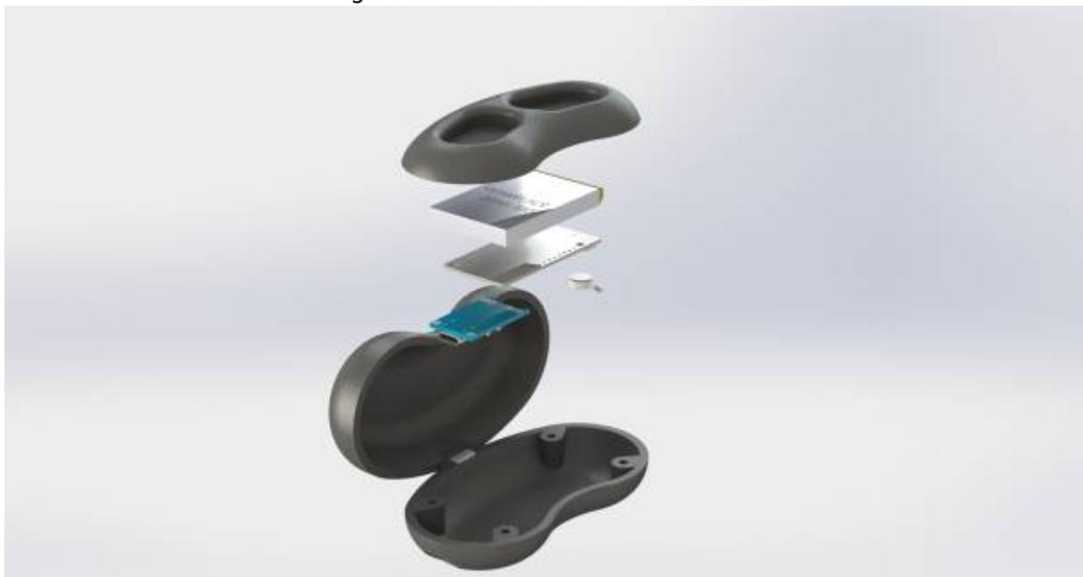
Figure 54: Exploded view of the smart case
