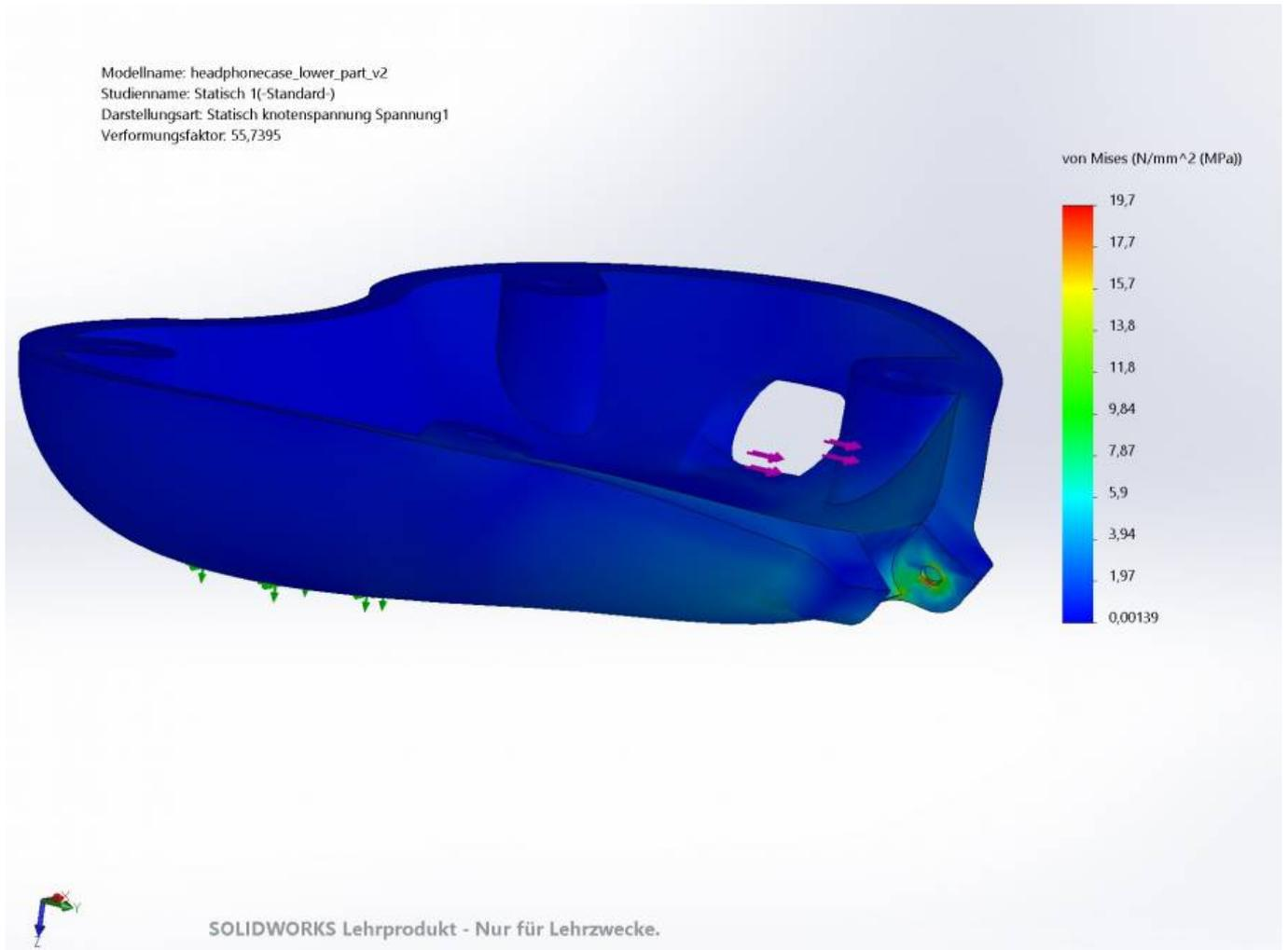
Figure 46: Stresssimulation Headphonecase Lower Part 1
